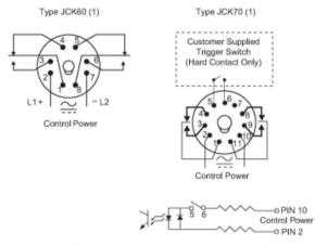
(1) Do not apply DC voltage to the 240 Vac timers (voltage code V24).
